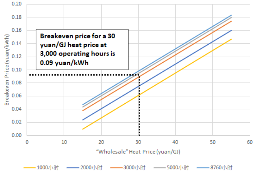
Figure 2. Breakeven electricity price for electric boilers (y-axis, yuan/kWh) as a function of wholesale heat price (x-axis, yuan/GJ), at different annual operating hours for the electric boiler (lines)
