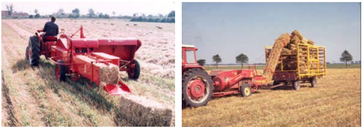
Figure 2.8. Light machinery for producing small bales of 12 kg (Nielsen 2003)
