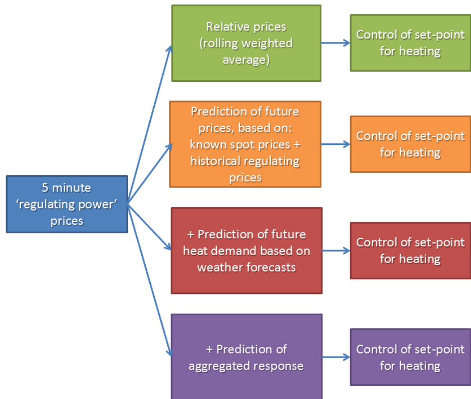
Figure 25: From the simple to the advanced, future potential development paths for electric heating guided by price signals.
