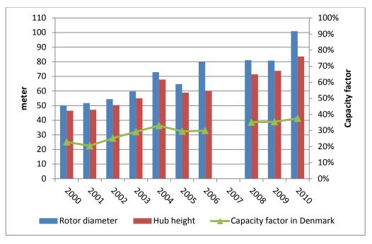
Figure 1: Development in average rotor diameter, hub height and capacity factor for onshore wind turbines commissioned in Denmark between 2000 and 2010 based on generation data for 2010. (No turbines commissioned in 2007)
