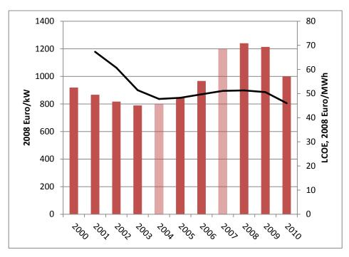
Figure 2: Average costs per kW for wind turbines commissioned in Denmark (columns) compared to development in average LCOE for wind power projects commissioned in that year (line) in Denmark. Data for 2004 and 2007 are estimates based on offers made to developers as no project cost data could be accessed for commissioned projects.
