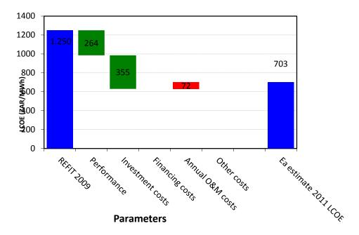
Figure 4: Influence of different parameters on LCOE for wind power in 2011 compared with REFIT 2009. The green columns indicate parameters that have reduced the 2011 LCOE compared with REFIT 2009, whilst the red columns indicate parameters that increase LCOE 2011 compared to REFIT 2009.
