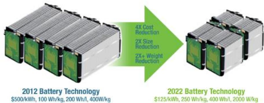
Figure 11: Battery advancement targets in the DOE's EV Everywhere Grand Challenge Blueprint (US Department of Energy, 2013a).
