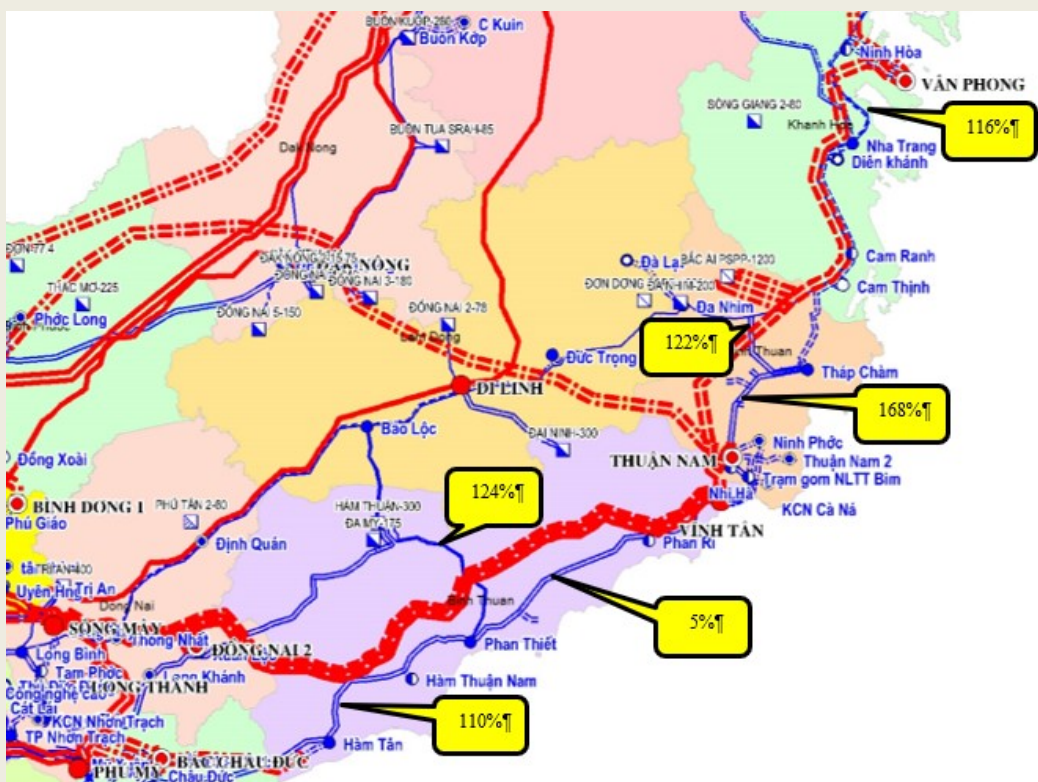
Figure 15 Overloaded elements in South Central in HWS snapshot for the C1 RE target scenario
