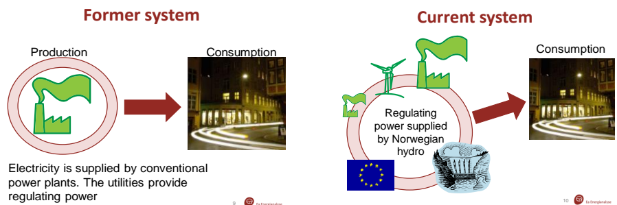
Exhibit 5: Nordic system development from 1980's to today where electricity is produced by many sources including wind power. The system is balanced to a large extent by means of Norwegian and Swedish hydro power.
