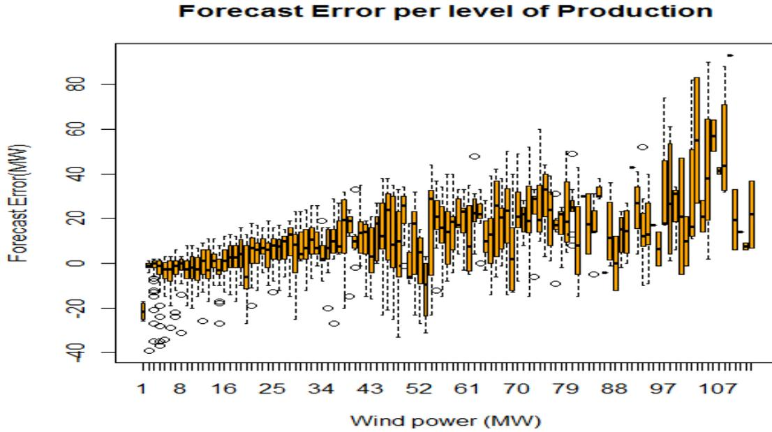
Figure 4.6: Plot of forecast errors compared to levels of wind production
