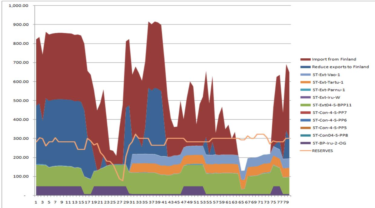
Figure 4.12: Results produced by BALMOREL for reserves compared to reserves calculated with the  $3\sigma$  method, 2013
