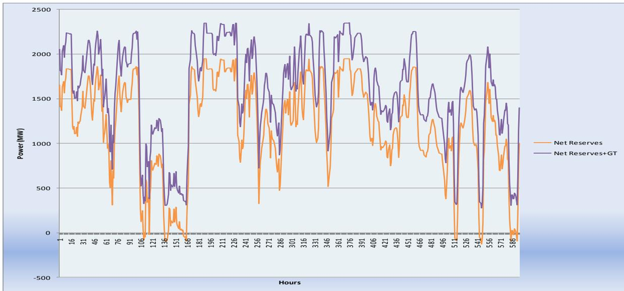
Figure 4.14: Net Reserves (Calculated reserves minus BALMOREL unused capacity) for 2016, with and without a 400 MW gas turbine
