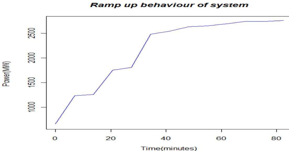
Figure 4.15: Ramp up rate of power system for Island case with all units running on minimal capacity, Estonia 2015
