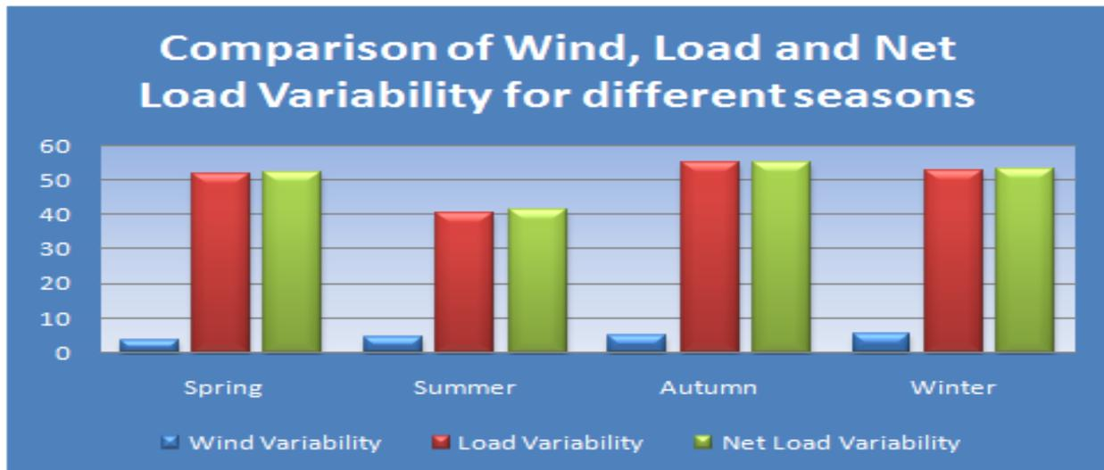
Figure 4.4: Standard Deviation of wind, load and net load for the different seasons of the year, Estonia 2007-2009
