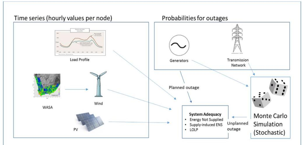
Figure 2. Outline of the computation in SisyfosR. Also hydro plants and pumped hydro may be represented by time series due to their limited / time-specific generation.
