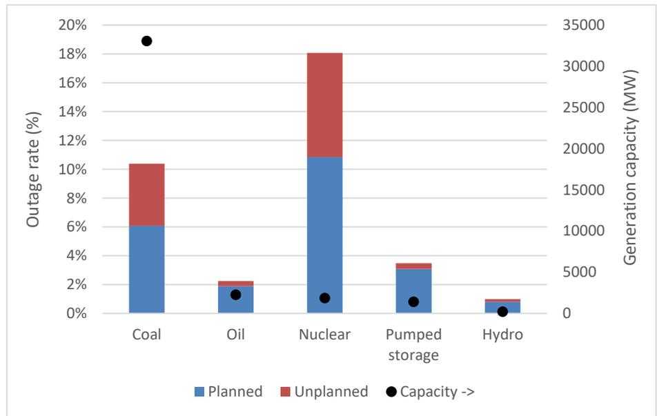
Figure 11. Average outage rates, 1998-2014, capacity-weighted. The total generation capacity per fuel type is shown on the right axis
