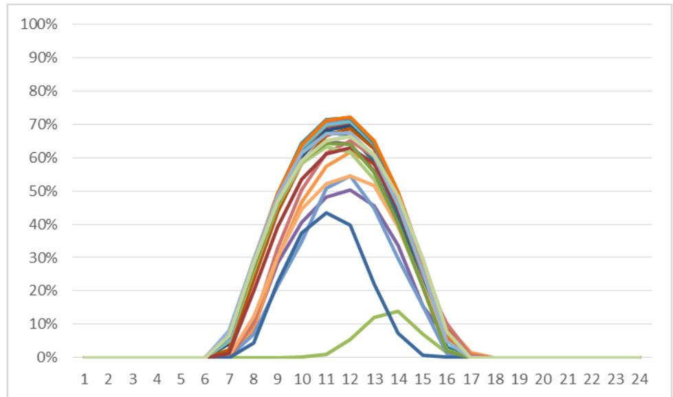
Figure 10. Examples of solar profiles for a specific day: 1 July. 27 nodes with PV capacity in 2020.
