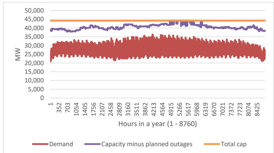
Figure 14: Demand, total generation capacity and capacity minus planned outages for the SisyfosR modelled year 2014
