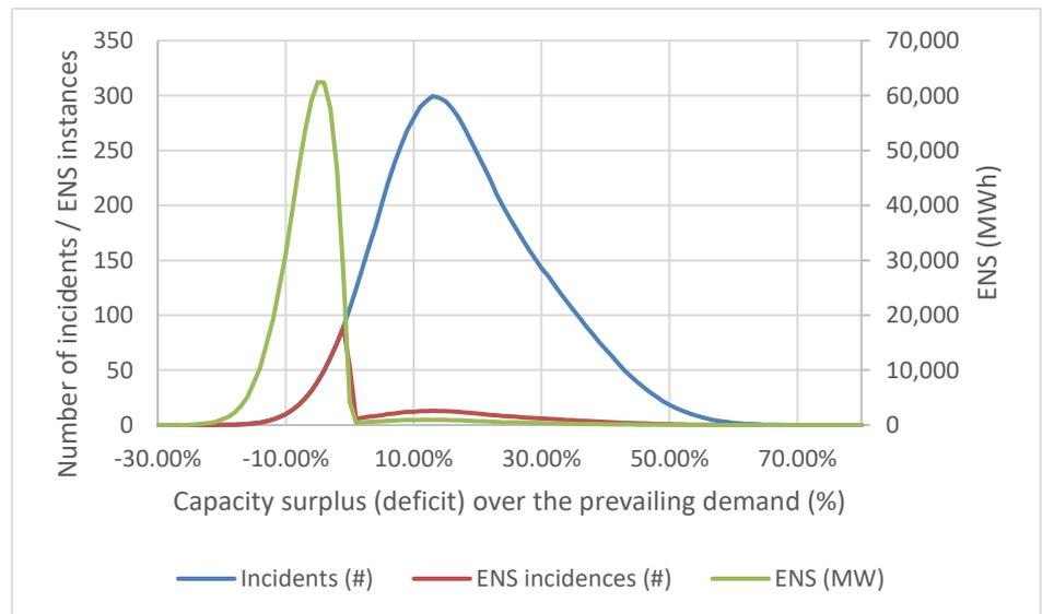
Figure 18: Histogram of average number of Incidents and ENS instances, as well as average ENS, over capacity surplus bins over the prevailing demand across the 1000 runs in SisyfosR for modelled year 2014
