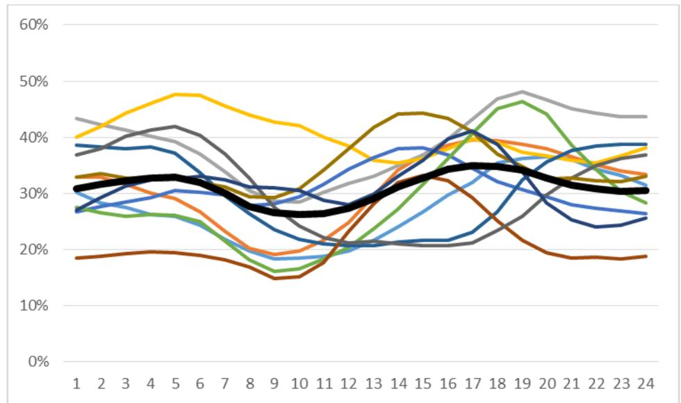
Figure 7. Yearly average wind generation across the hour of the day. Percentage of installed capacity. The black thick line is capacity-weighted average. The other lines are node-specific data.
