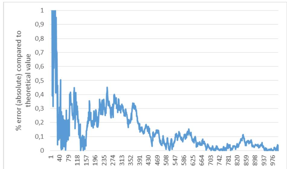
Figure 4. The SisyfosR result accuracy compared to the theoretical result. Results from a test with 1,000 runs.
