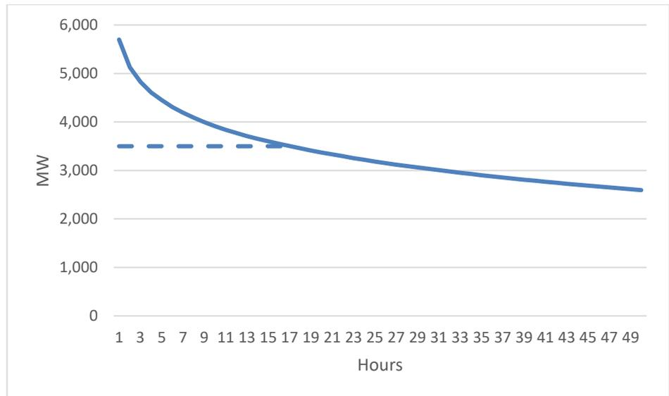
Figure 21. Duration curve for ENS. Data for 2014, with 1,000 MW capacity reserved for N-1 incidences. Assuming additional 3,750 MW, the area below the dashed line will be avoided as ENS, However, the area above the line will still be ENS.
