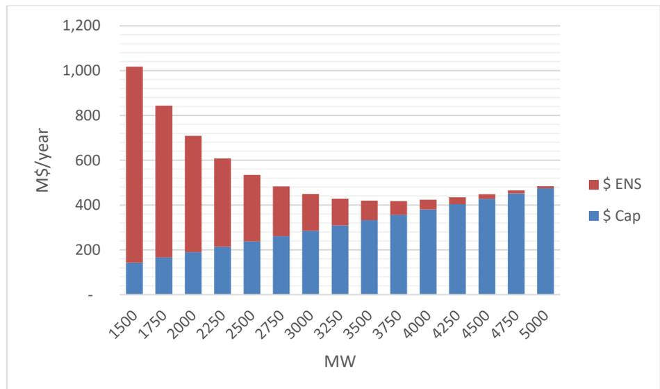
Figure 22. Total cost for ENS (red) and new capacity investment (blue). Minimum total costs can be found at 3,750 MW of new capacity.
