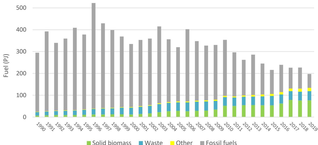
Figure 1: Development of fuel consumption for electricity and district heat production 1990 - 2019.
