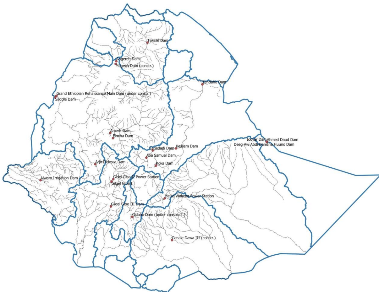
Figure 8: GIS map with basin areas in Ethiopia and the locations of hydropower plants
