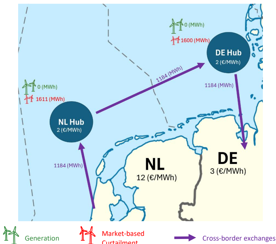
Figure 15: Electricity price and flows around the hubs in question, in the OBZ case during week 38, hour 154
